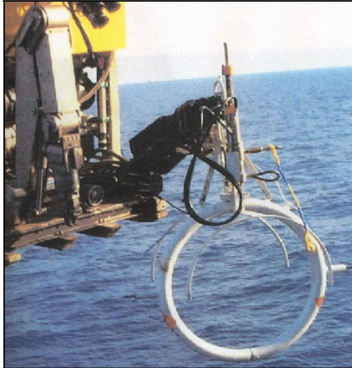
Figure 1-14. Externally-Deployed LSC Mounted to ROV (JRC, 2002).
