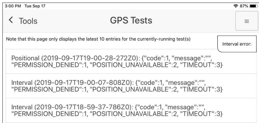
Figure 98: Positions unavailable during the GPS Testing
