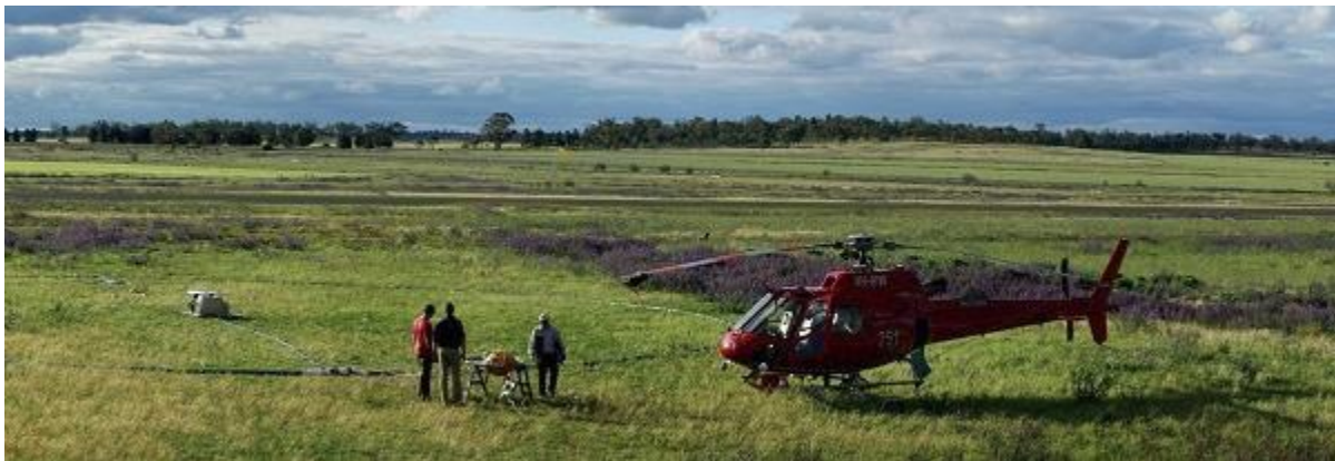
Figure 5 Rotor Wing Aircraft Used to Collect Gravity and Magnetic Data.
