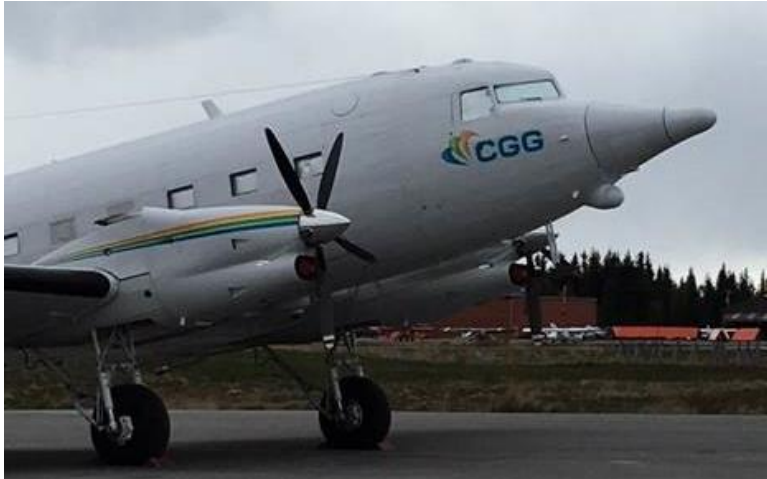
Figure 4 Fixed Wing Aircraft Used to Collect Gravity and Magnetic Data
