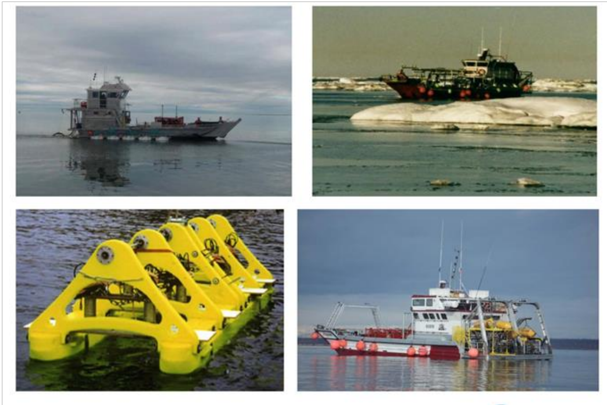
Figure 2: Source Vessels and Seismic Source Array
