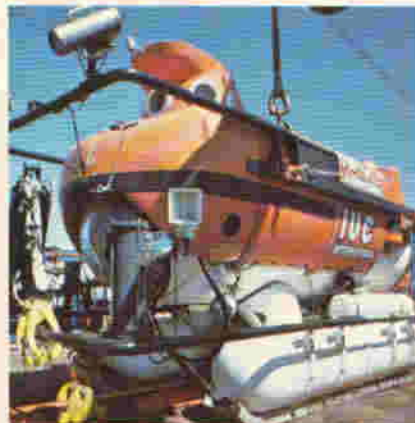
Aft-deck showing hydraulic crane launching IUC's 1,000-foot (305-meter) submersible Mermaid II.
