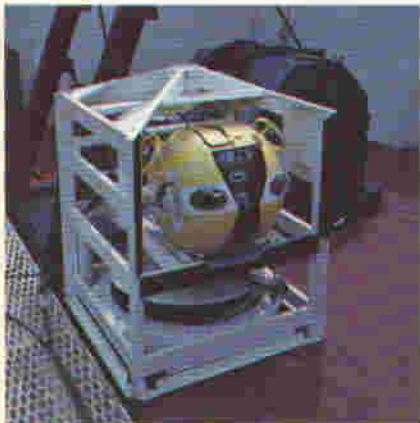
Aft-deck showing installation of IUC's-Hydro Products RCV 225 remote controlled underwater vehicle
