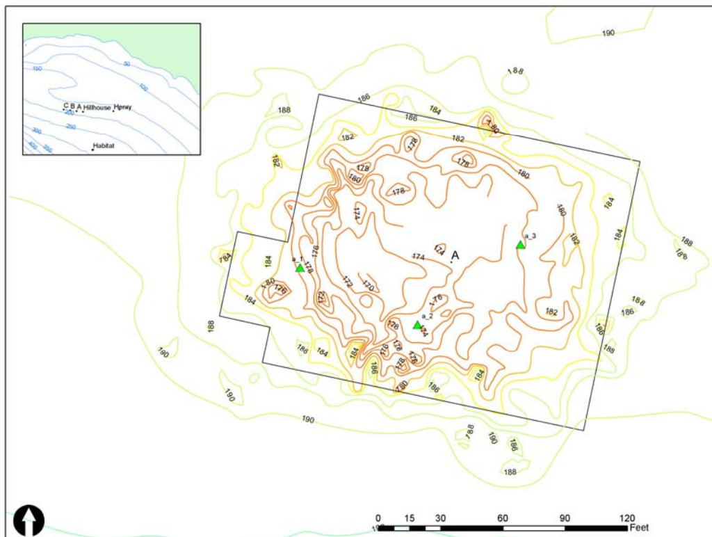
Figure 13. Side scan bathymetry beneath platform A with location of potential sampling locations indicated (green triangles).
