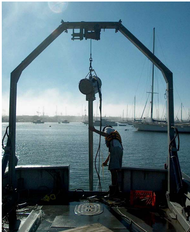
Figure 7. Photo of representative electric vibracore
