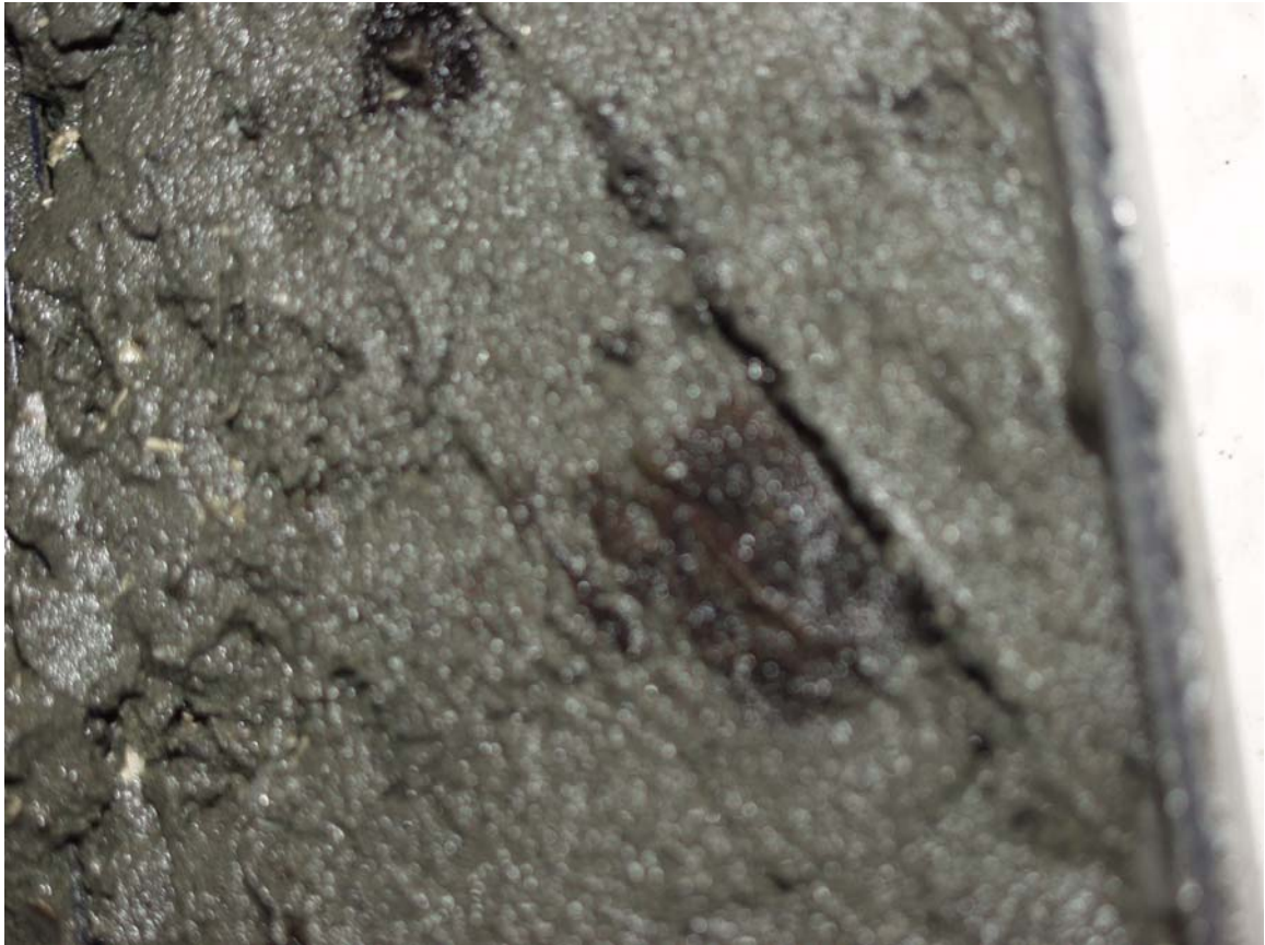
Gina – 1: Depth Interval; 5.5 feet (close up of small brown deposits, approx. 2 – 10 mm).
