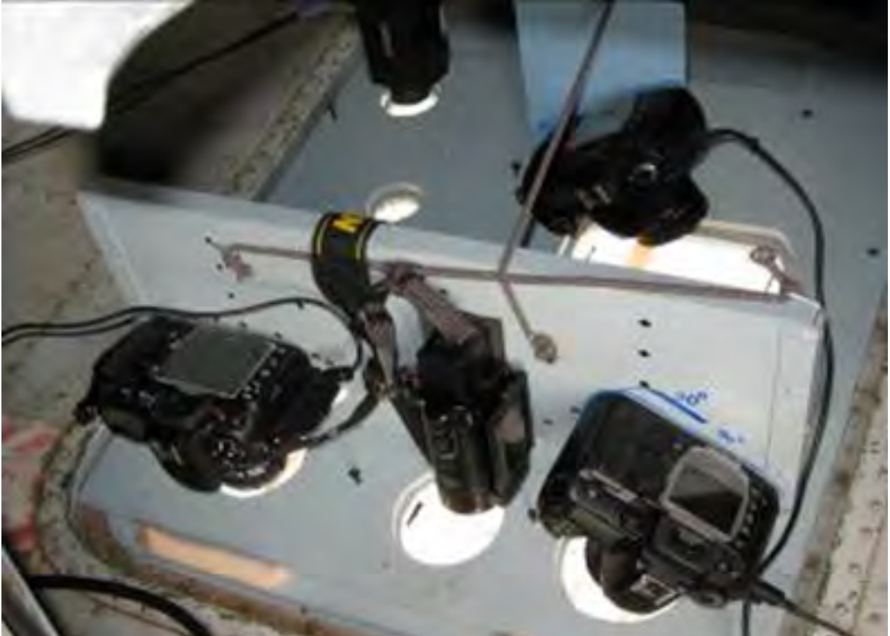
Figure 15. Russian survey aircraft camera setup showing a downward facing Nikon D3X and two oblique Nikon D300s. The cooled thermal imager, Malahit-M, is in a separate compartment of the aircraft.
