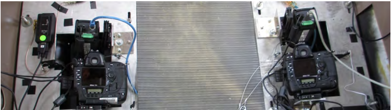
Figure 14. Aero Commander instrument setup. A Nikon D3X digital SLR camera paired with a FLIR SC645 thermal imagers, in each of two belly ports.
