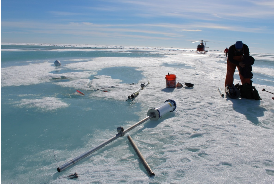
Figure 6. Ice conditions at the site of IceTracker 0016 on May 23, 2015. Significant surface melting had taken place between deployment and the time that this picture was taken. There was no river overflowing present at the location of the IceTrackers (as indicated by MODIS imagery and CTD measurements taken at the same time as the photo above).
