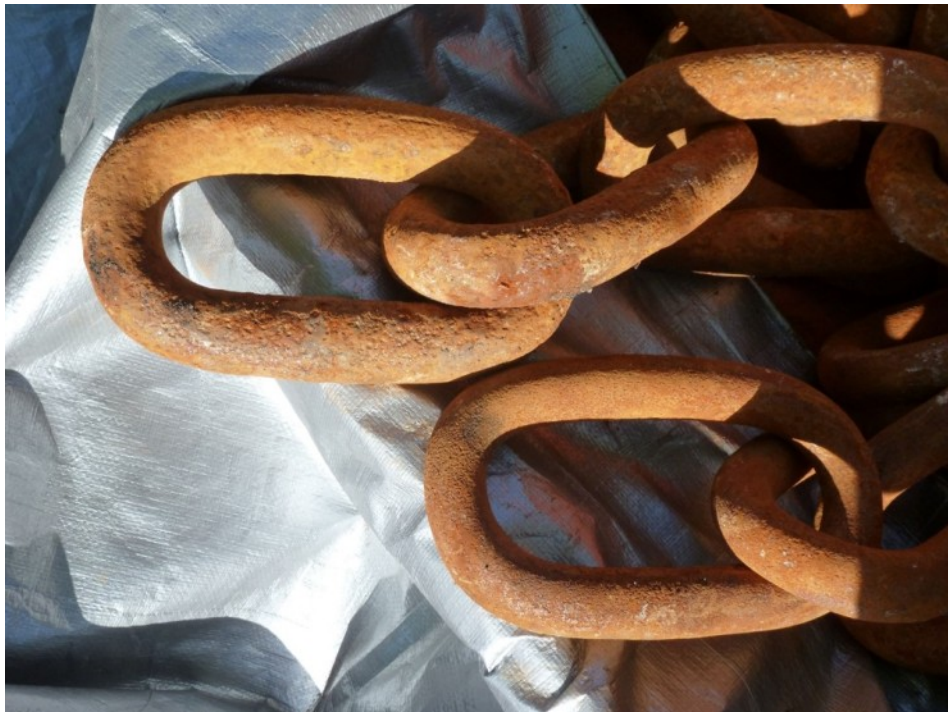
Figure 21: 1.5" chain samples from the Marshall Point buoy. The lower sample is from the chafe zone.
