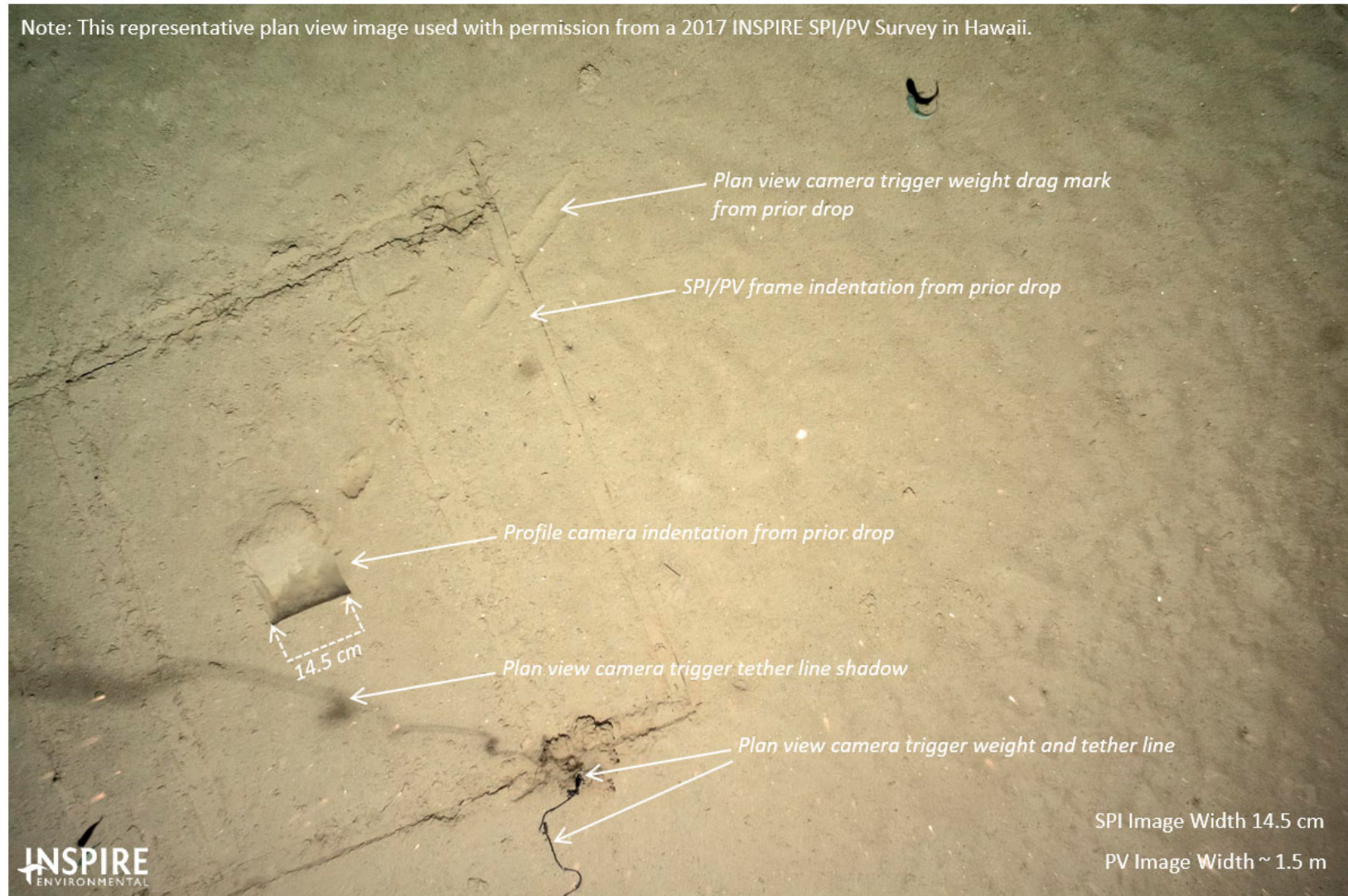
Figure 2-2. This representative plan view image shows the sampling relationship between plan view and sediment profile images. Note: plan view images differ between surveys and stations and the area covered by each plan view image may vary slightly between images and stations.
