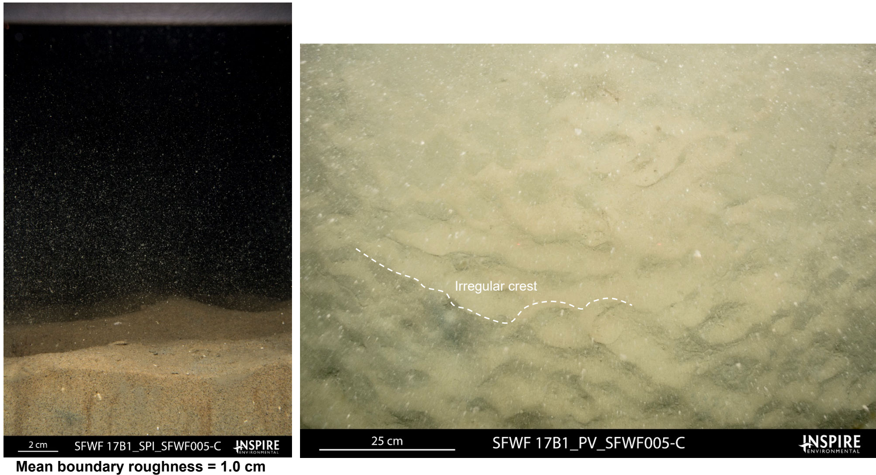
Figure 3-15. Representative SPI and PV images from Station 5 showing mobile fine sand with irregular short period ripples. Shallow boundary roughness and short (~4-10 cm) ripple periods and anastomosing or sinusoidal crests are evidence for this bedform.
