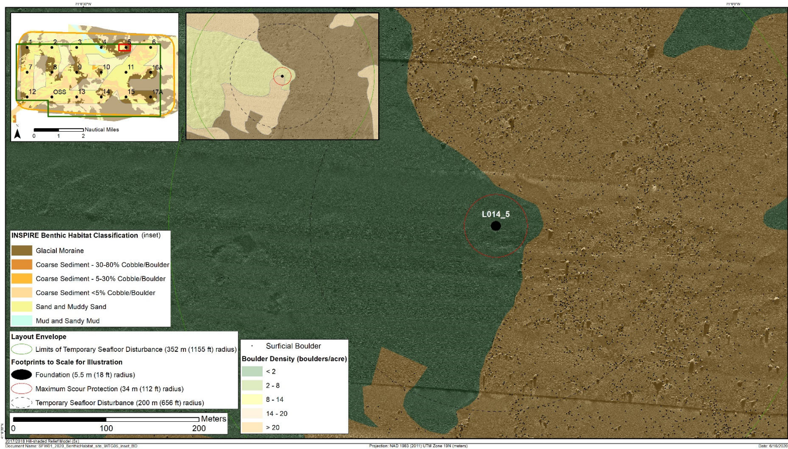
Figure 4-6. WTG-5 footprint with habitat classification, boulder density, and high-resolution side-scan sonar
