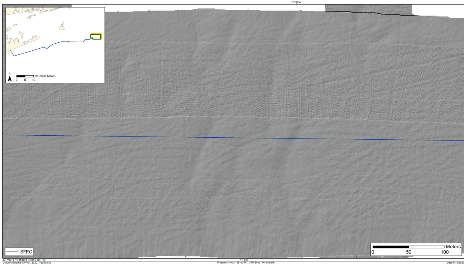
Figure 3-17. Trawl marks visible in hill-shaded bathymetric relief model along the SFEC – OCS
