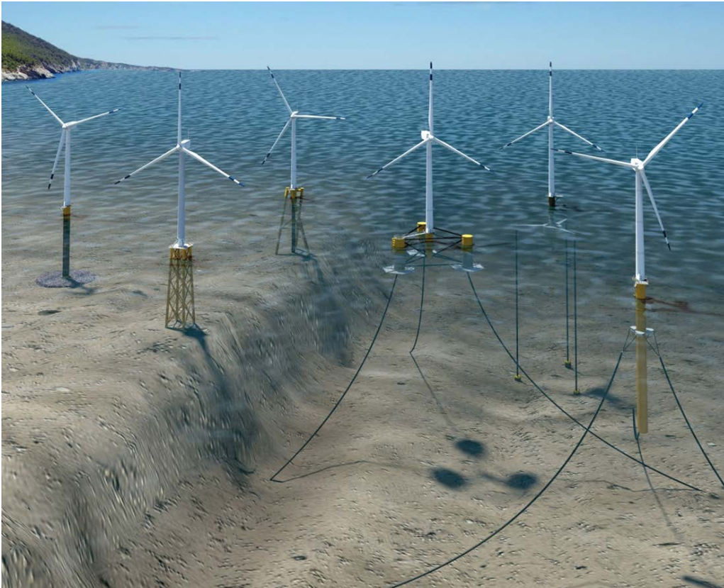
Figure 1. Offshore wind substructure designs for varying water depths (Illustration by Josh Bauer, NREL)
