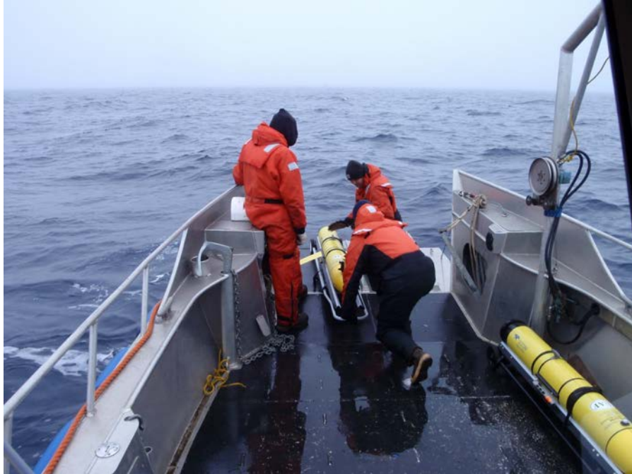
Figure 6. Two Webb Slocum gliders being deployed in the northeast Chukchi Sea off the Wainwright-based vessel Tukpuk in 2010.
