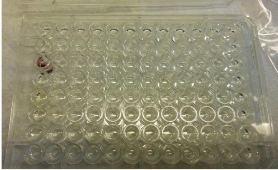
Figure A3. MPN plate for C2S1 and C2S2 samples at 3°C with diesel as C source.
