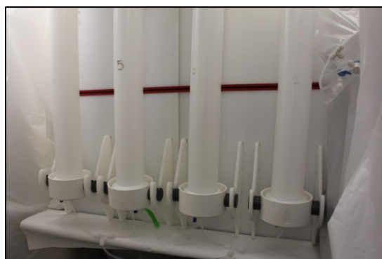
Figure 4. Custom-made chambers for melting sea ice cores. Chambers can be outfitted with individual filter discs to capture particles released by the melted ice or linked with tubing to collect a single homogenized sample.
