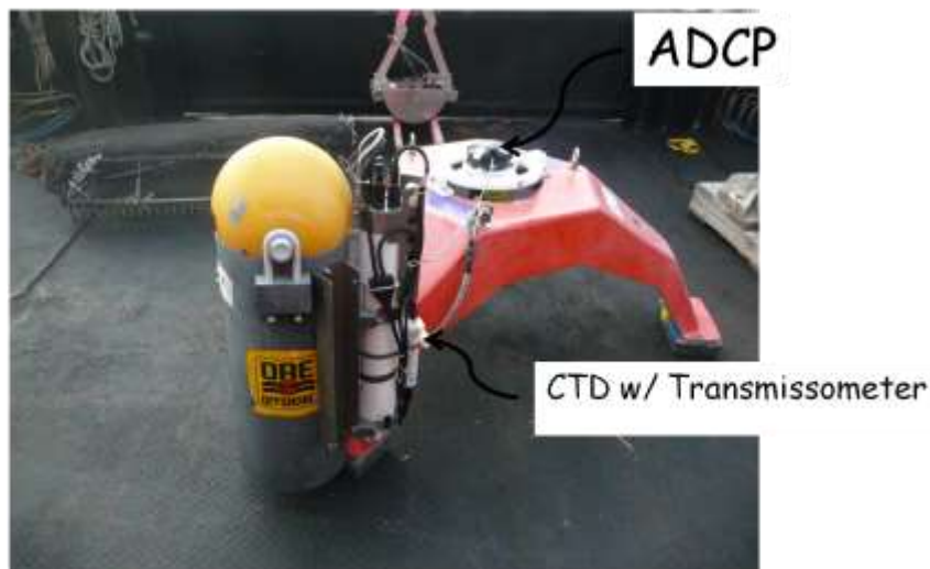
Figure 4. Physical oceanographic mooring deployed in Harrison Bay.
