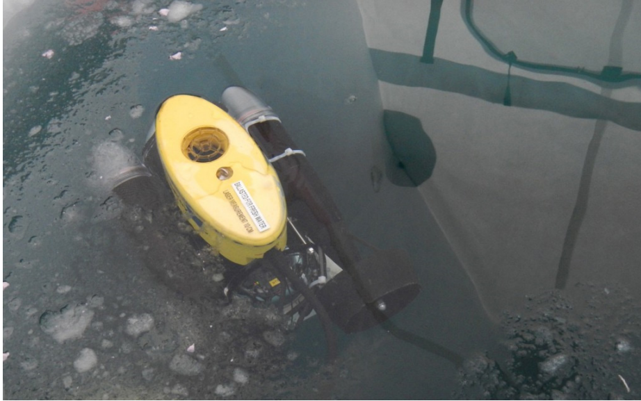
A remotely operated vehicle (ROV) deployed under ice can provide live video feed. Photo by Lorena Edenfield.
