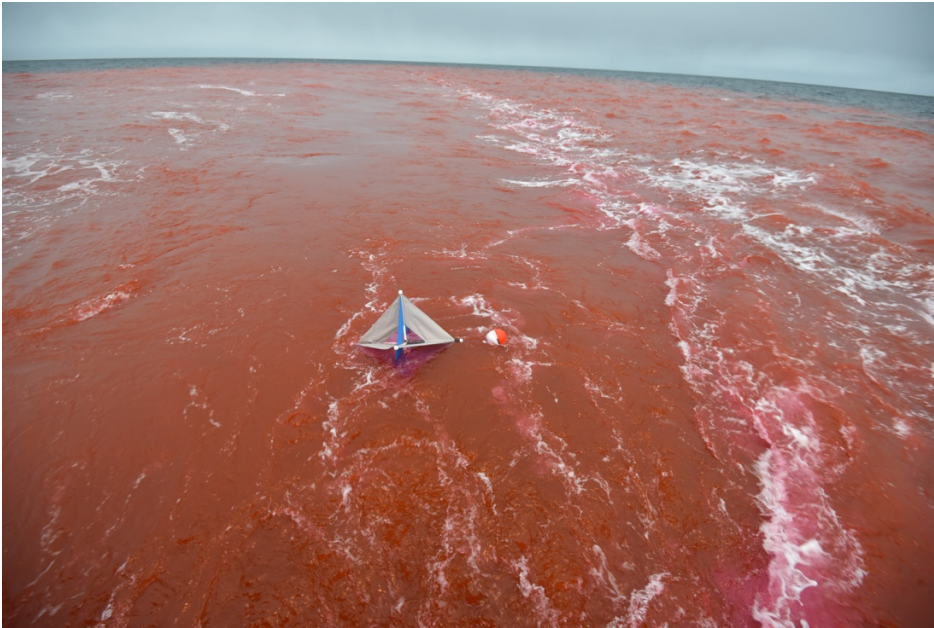
Figure 2. Photo of a surface Rhodamine-WT dye injection, Chukchi Sea. Visible in the center of the picture is a surface drifter that was just deployed off the aft deck of the R/V Norseman II . The drogue sank within 1 minute of deployment.
