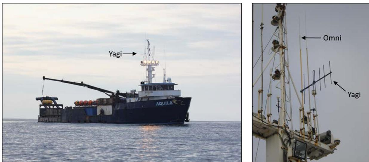
Figure 59. Omnidirectional and Yagi antenna placement (A) in relation to the R/V *Aquila* and (B) in relation to each other on the crew's nest.
