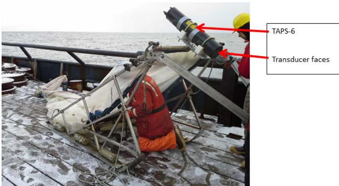
**Figure 85.** 1 M<sup>2</sup> Tucker sled on the icy deck of the R/V *Aquila*. The kneeling scientist has his head in the net mouth. The TAPS-6 (black canister) is mounted on the top bar of the tucker frame and is pointed down into the tow path of the net. The transducer faces point to the right and down in this picture.
