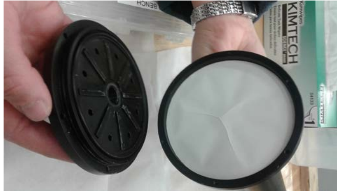
Figure 9: Picture of the wrinkled membrane from prototype 2.1 following successful sawtooth and hover missions during the August 2016 sea trials.
