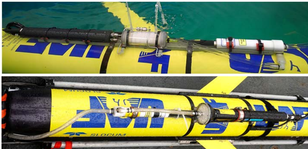
Figure 2. Carbon glider with prototype 1.1 (upper panel) and 2.1 (lower panel) p\text{CO}_2 sensors. The prototype 1.1 configuration (upper panel) includes an SBE 5P pump.
