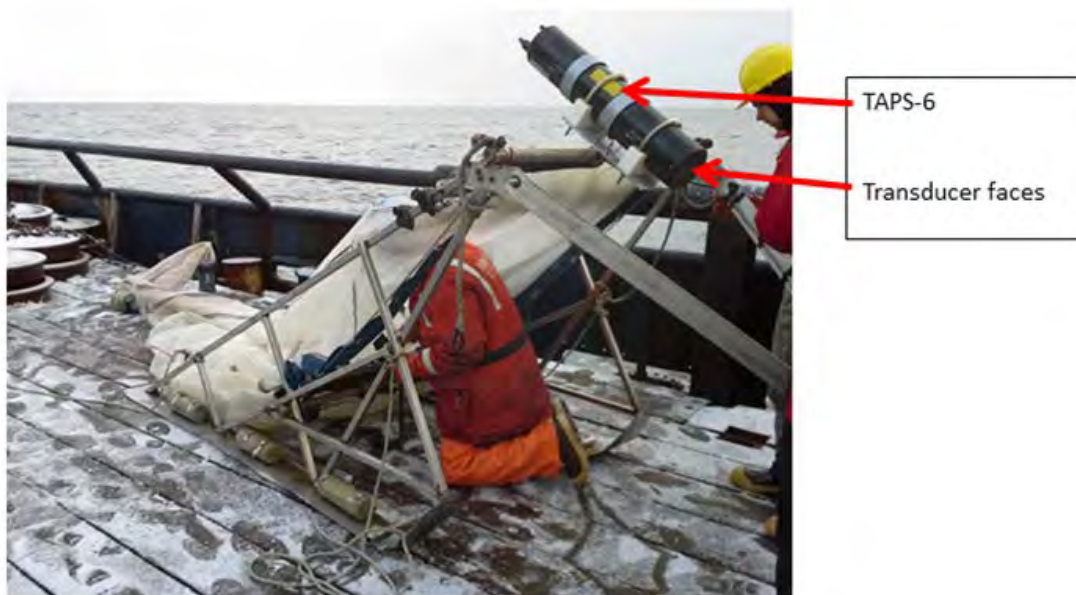
Figure 145. 1 m 2 Tucker sled on the icy deck of the R/V Aquila. The kneeling scientist has his head in the net mouth. The TAPS-6 (black canister) is mounted on the top bar of the Tucker frame and is pointed down into the tow path of the net.
