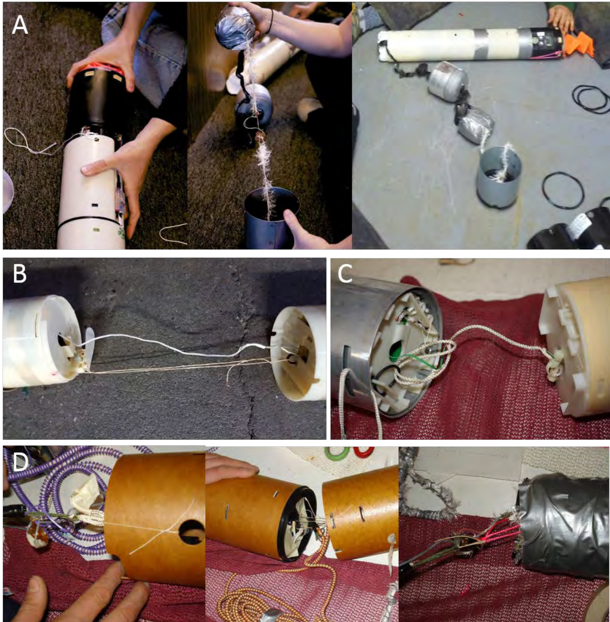
Figure 92. A) Modifications of a 77C (SPW) sonobuoy (top row, left to right): Tying up the top housing; taping up the bottom array of sensors; a 77C sonobuoy fully modified. B) Modifications of a 53 F (USS) sonobuoy to shorten deployment depth by tying the main spool housing to the top float to prevent cable from unspooling. C) Modifications of a 53D (USS) sonobuoy to shorten deployment depth by tying the main spool housing to the top float to prevent cable from unspooling. D) Modifications of a 77B (MAG) sonobuoy (bottom row, left to right): Tying the elastic cable to the middle housing; tying the float to the top housing to prevent spool of cable from deploying; taping up the bottom array of sensors.
