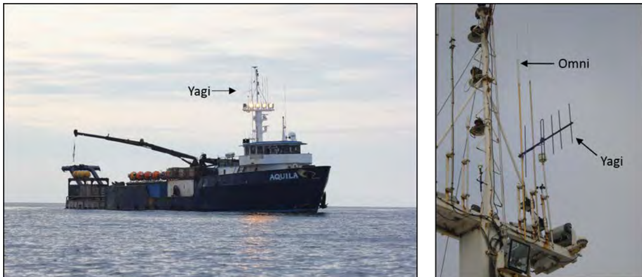
Figure 94. Omnidirectional and YAGI antenna placement (left) in relation to the R/V Aquila and (right) in relation to each other on the crew's nest.
