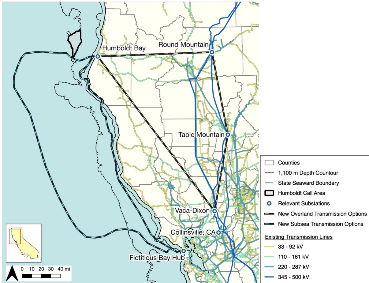
Figure A-16. Transmission upgrade alternatives for 1.8 GW of offshore wind from the Humboldt Call Area.
