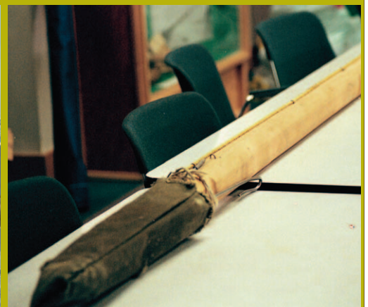
Whaling harpoon with sleeved bomb mechanism
