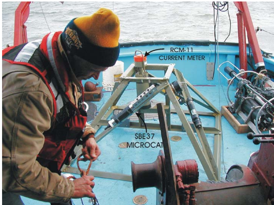
Figure 2 Eluikak Pass (Barrow) current meter mooring on the afterdeck of the R/V Annika Marie after recovery.
