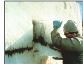
Oil Encapsulated in ice during an experimental spill in Alaska. Photo: A. Allen
