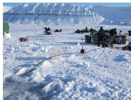
3400 litres of Statfjord crude pumped under 65 cm ice
