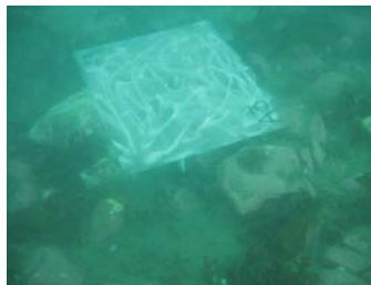
Figure 4. Settlement plate at DS-11.
