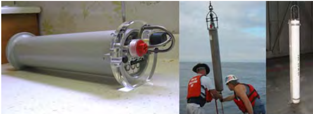
Figure 8: Three types of passive acoustic recorders used. A) Ecological Acoustic Recorder (EAR); B) Haruphone; C) Autonomous Underwater Recorder for Acoustic Listening (AURAL).
