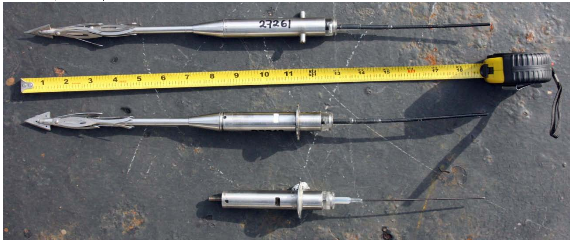
Figure 5: SPOT 5 satellite transmitters deployed on NPRWs in the SEBS in 2008 and 2009.
