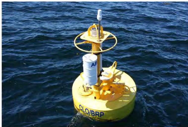
Figure 2. An above-surface view of the automatic detection buoy deployed in the Bering Sea.
