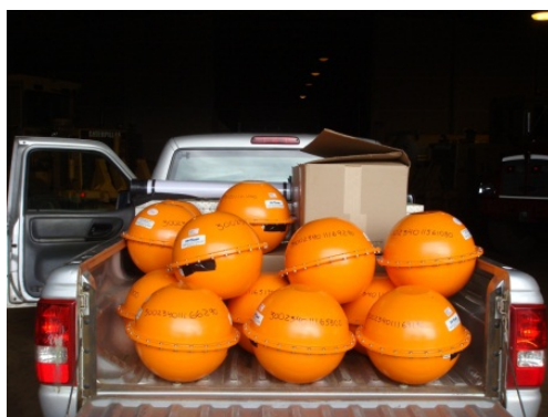
Figure 2. The iSphere surface drifter manufactured by Metocean.
