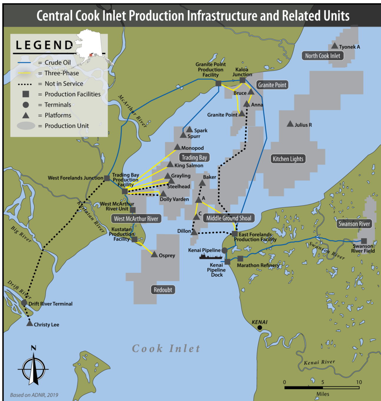
Figure 2. Cook Inlet oil and gas production infrastructure and related units
