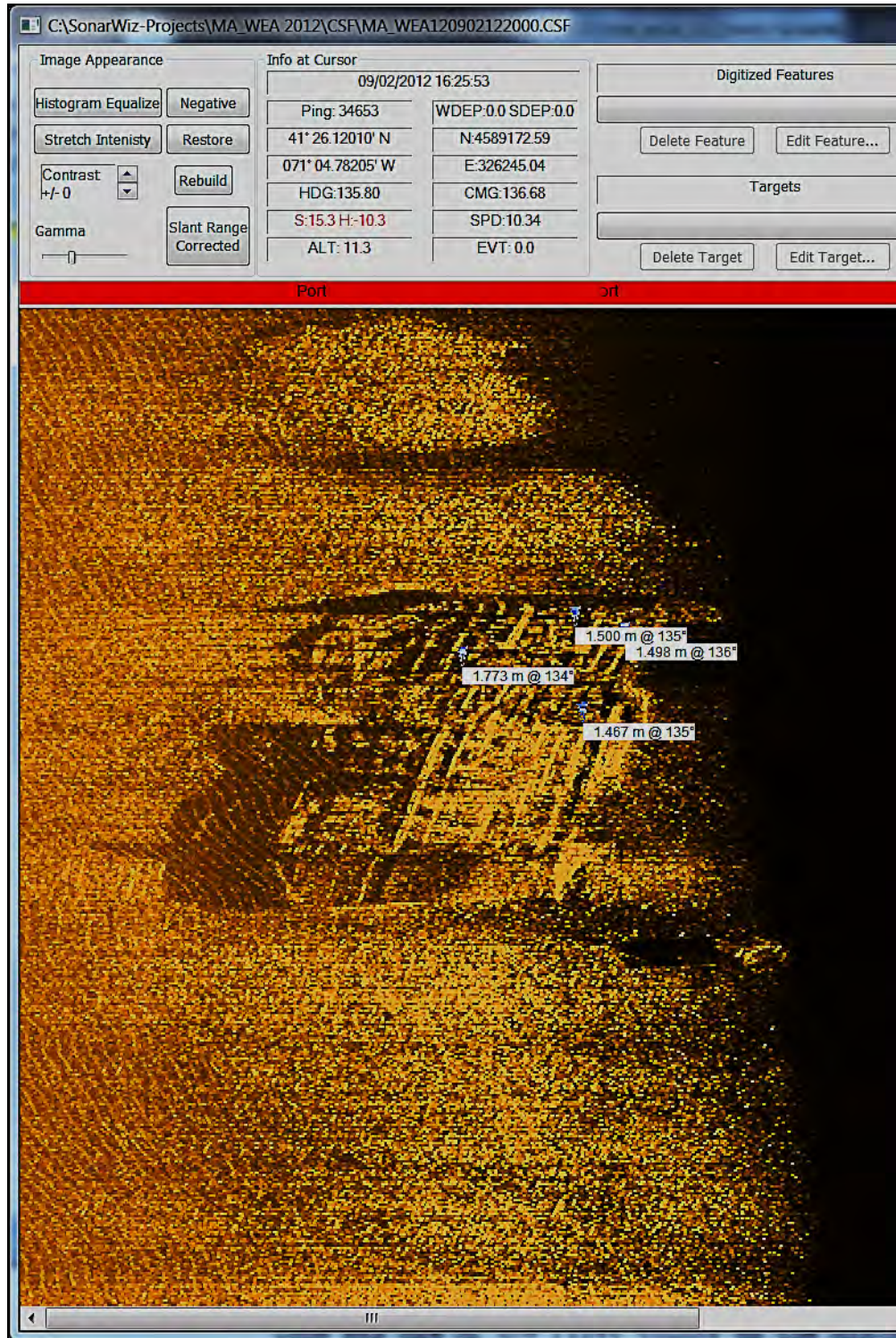
Figure 6-11. Transverse resolution of 900 kHz data on parallel features of shipwreck. Bearings in degrees indicate direction of measurement.
