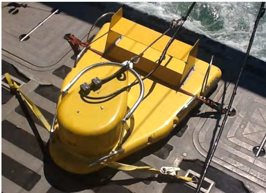
Figure 1-4. The towfish of the EdgeTech 3200 SB-0512i sub-bottom profiler aboard the R/V SRVx.
