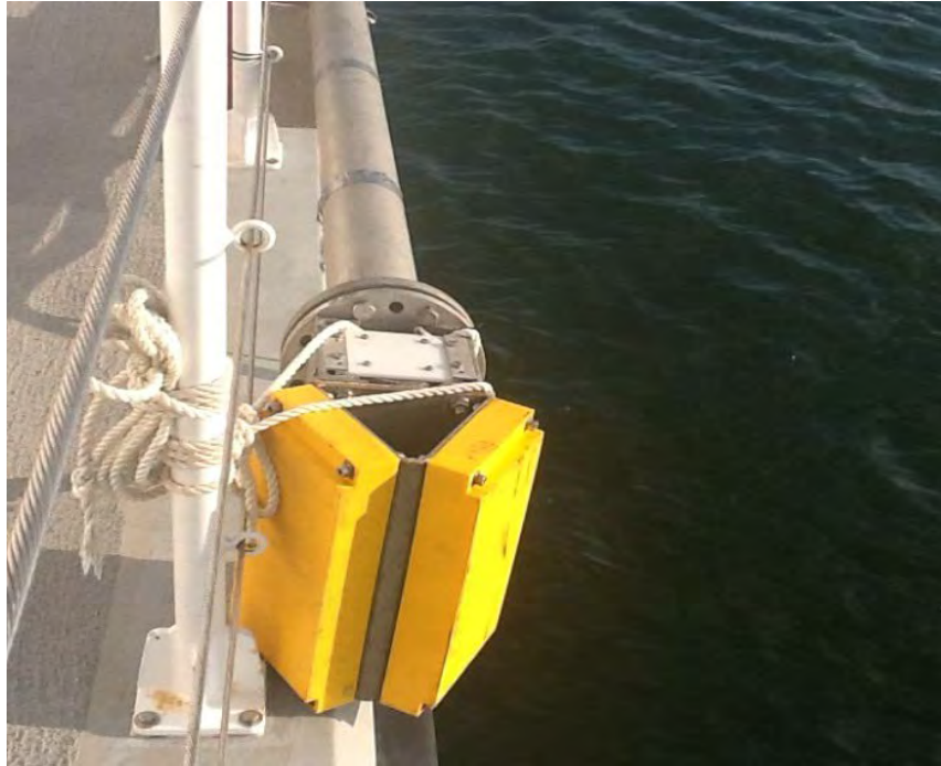
Figure 7-2. The SEA SWATH plus -M interferometric sonar (Systems Engineering & Assessment Ltd.) before deployment from the R/V SRVx in Rhode Island Sound.
