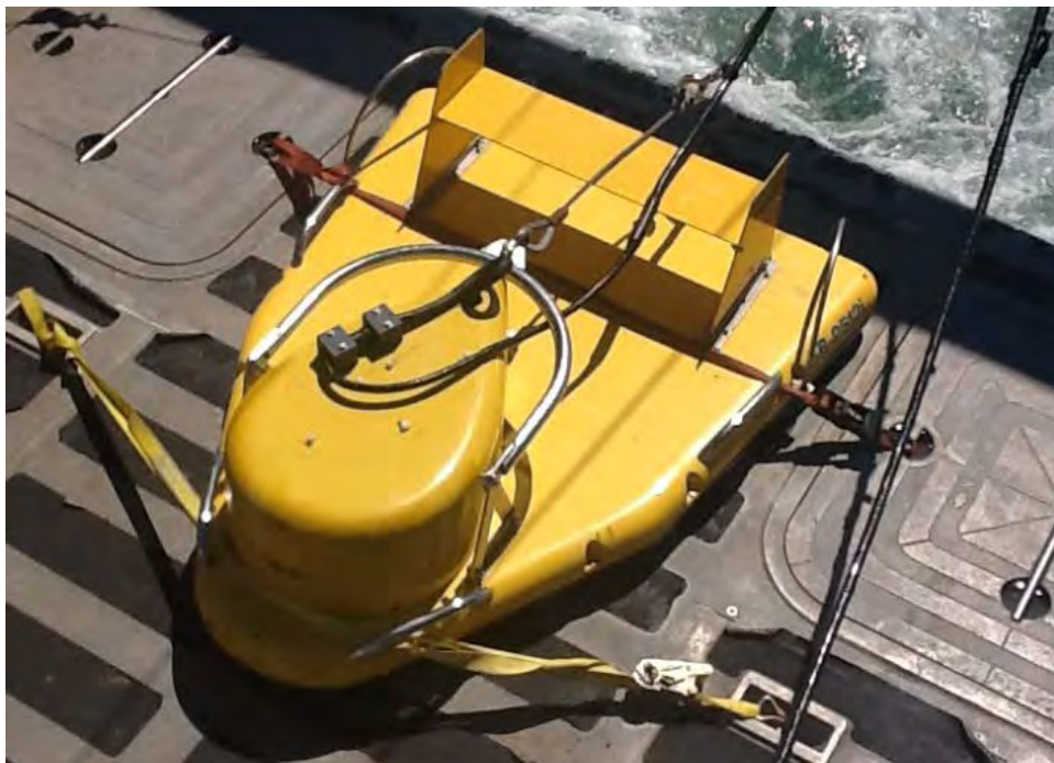
Figure 7-3. The towfish of the EdgeTech 3200 SB-0512i sub-bottom profiler aboard the R/V SRVx.
