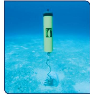
FIGURE 4. WILDLIFE ACOUSTICS' SM2M MARINE RECORDER WHICH RECORDS UNDERWATER SOUNDS
