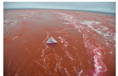
Surface drifter moving in a pool of Rhodamine-WT dye in the Chukchi Sea, by Dr. Peter Winsor, from the aft deck of the Norseman II in 2015.
