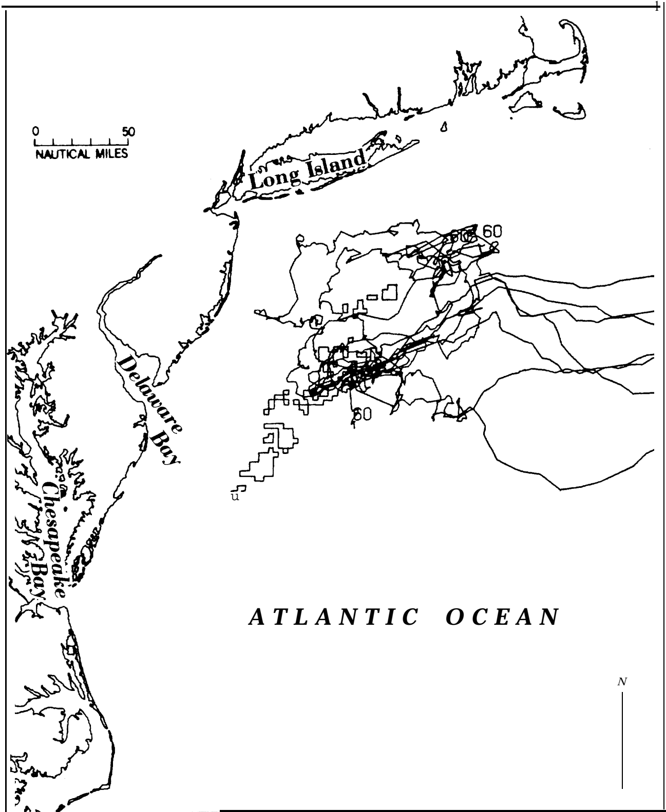
FIGURE 8.—Example oilspill trajectories for a spill site (P4) near the center of the proposed Mid-Atlantic (OCS Lease Sale 49) lease area: summer conditions. Number on trajectory is the time to the end point in days. (Slack and Wyant, 1978. )
