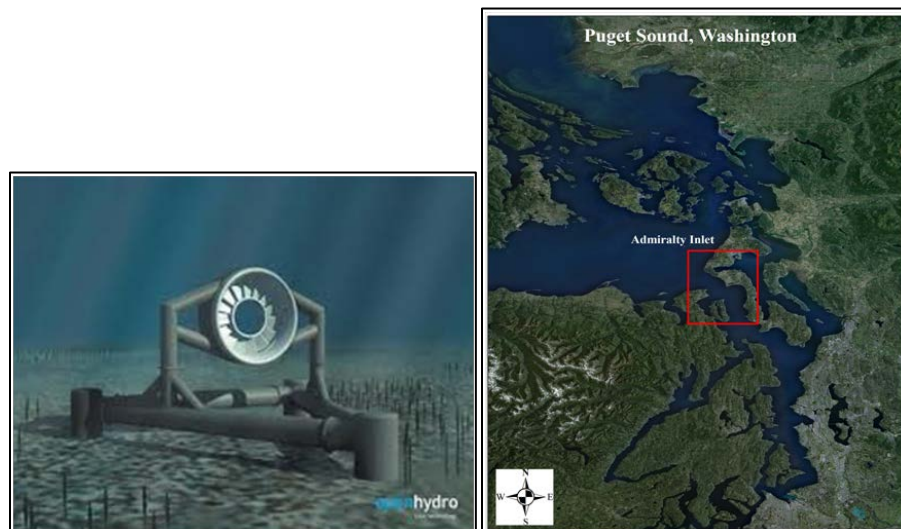
Figure 6-1. Open Hydro Turbine and Project Map. Left: Schematic of an open-center OpenHydro turbine. Right: Map of Puget Sound, Washington, with commercial tidal project site in Admiralty Inlet denoted by red box.
