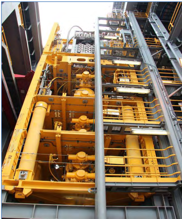
Figure 7. Example of a Typical 15,000-psi Subsea Blowout Preventer (BOP) Stack. New equipment has been developed with a rating of 20,000 psi. Source: USDOl, BSEE, pictured in Pallanich, 2017.
