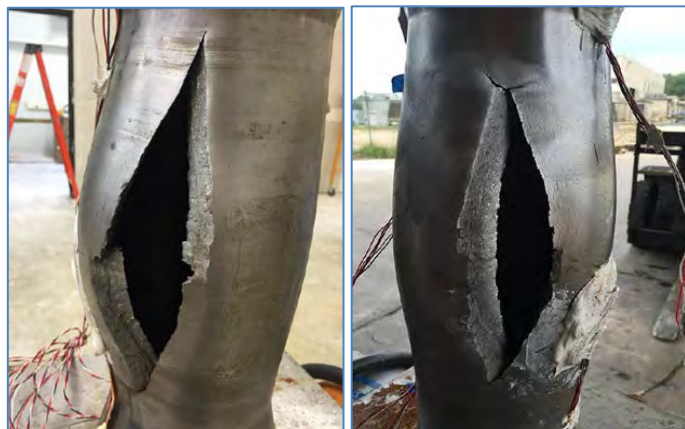
Figure 5. Examples of Ruptured Test Bodies from High-Pressure Testing. Source: Aiken, 2016.
