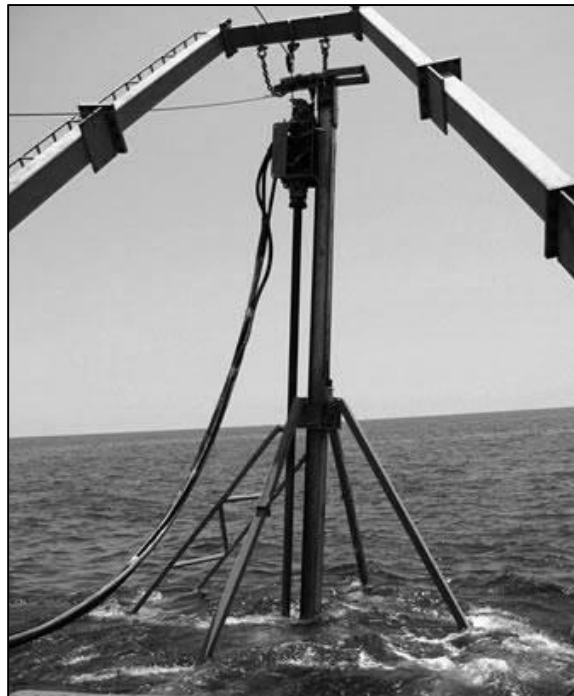
Figure 2-2. Deployment of a 20-foot Vibrocore from Stern A-frame
