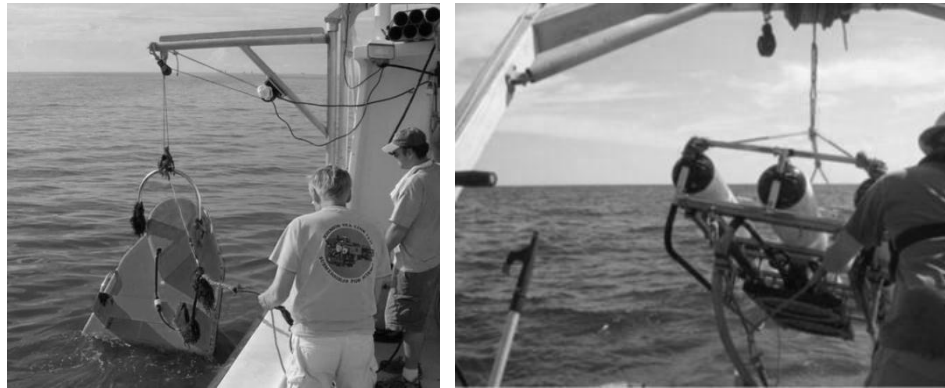
Figure 2-1. Deployment of Chirp towfish from Port Davit (left). Deployment of Boomer Sled from Stern A-frame (right).
