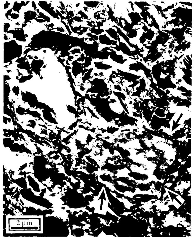
Fig.4. High-magnification view of BCF sediment. Domains (arrows) are wrapped around a shlorite grain (C). Pulverized or degraded microcrystalline chlorite (Cc) and fine clay-size domains (small arrows) comprise the matrix.
