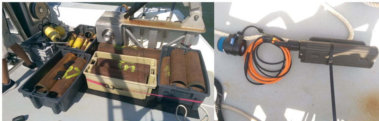
Figure 3: Munitions surrogates (left) were initially lowered on a slack-line with USBL puck (right) attached. The USBL was abandoned for the later deployments due to complications from a strong thermocline. Vessel GPS was used to mark the remainder of the surrogate positions.
