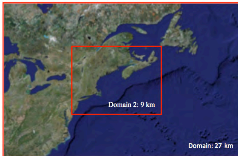
Figure 2.6: Illustration of the NECOFS-WRF domains. The output of the WRF model in domain 2 was used to drive GOM3-FVCOM and NS-FVCOM.
