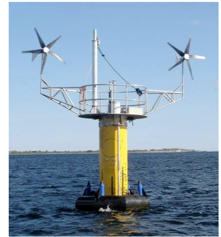
Floating wind LIDAR; The Natural Power Sea ZephIR (from http://blog.lidarnews.com )
