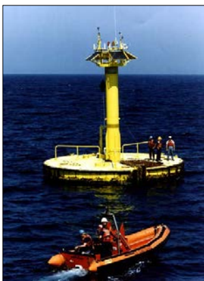
Figure 3-5(a) 10-Meter Discus-Shaped Hull Buoy
