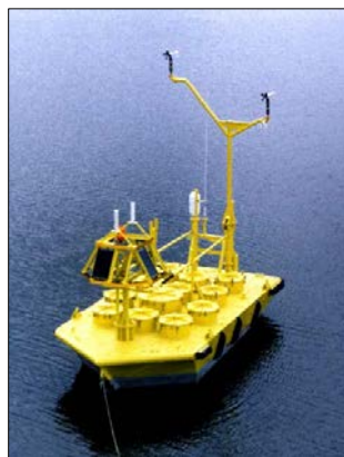
Figure 3-5(b) 6-Meter Boat-Shaped Hull Buoy
