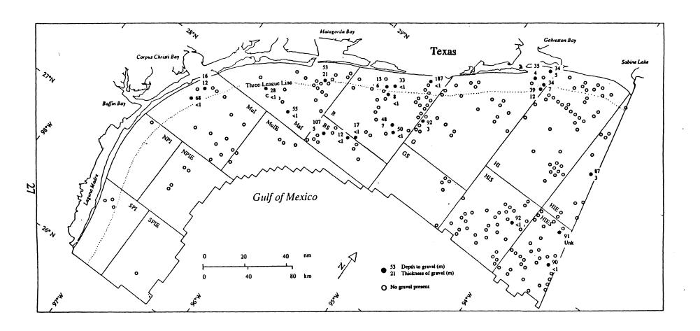
Figure 11. Distribution of foundation borings containing gravel. Depth below seafloor and thickness of gravelly strata included for borings that encountered gravel.
