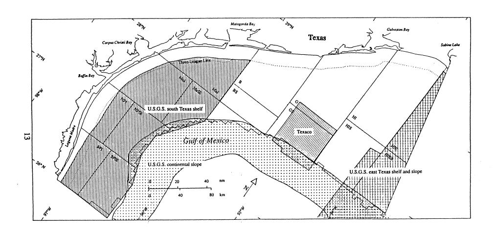
Figure 5. Location of high-resolution seismic surveys on the Texas continental shelf and slope.
