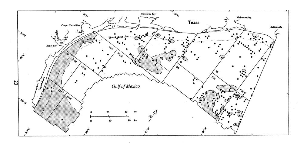
Figure 9. Distribution of foundation borings (shaded) containing more than 7.5 m of sand in the top 15 m of sediment below the seafloor.
