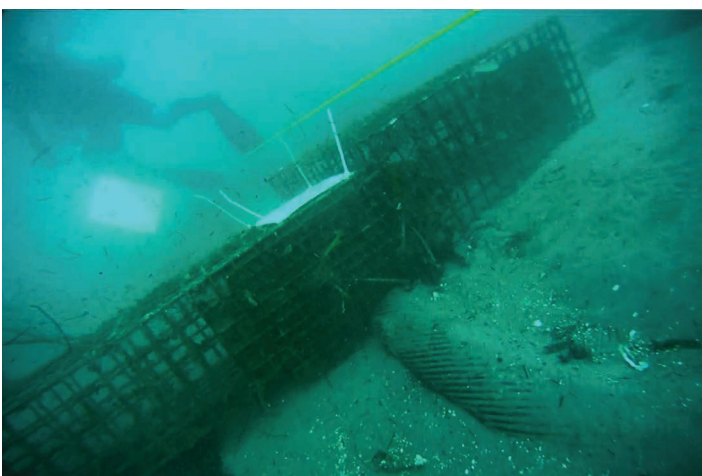
Experimental equipment used to test whether crabs will cross a seafloor power transmission cable to reach a baited trap. The apparatus, which includes a crab introduction chamber (lower left) and a baited trap (upper right), sits directly on top of the cable. Yellow rope guides divers to/from each apparatus in poor-visibility conditions. Photo by Brandon Doheny, University of California, Santa Barbara.
