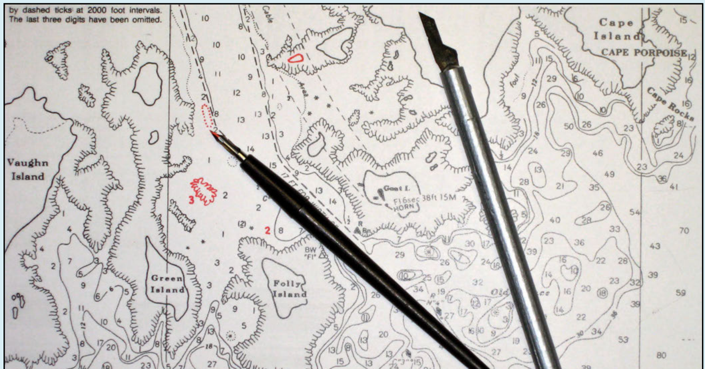
Mapping tools of the past included the crow quill pen (left) and the artist's knife (right).
