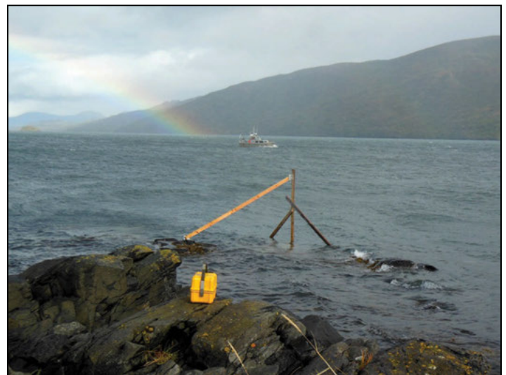
The new tide gauge staff installed at Kizhuyak Bay.
