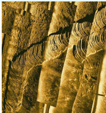
Side scan sonar mosaic showing scars on the seafloor from offshore dredging. From Research Planning, Inc. et al. 2004.
