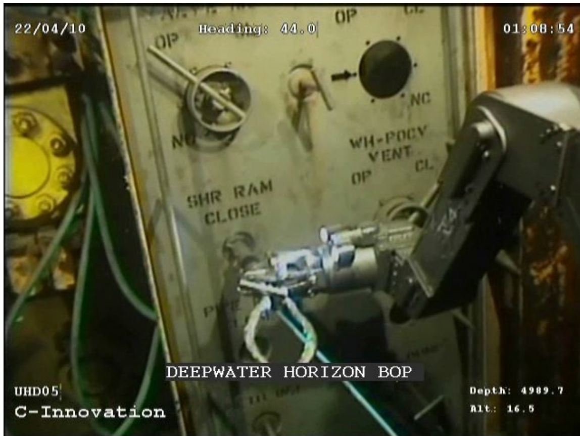
Figure 27: A robotic arm of a Remotely Operated Vehicle (ROV) attempts to activate the "Deepwater Horizon" Blowout Preventer (BOP), Thursday, April 22, 2010.
