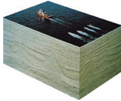
Photo 2. Typical Marine Seismic Survey Vessel and Towed Array Configuration and Seafloor Imaging Data (USDOI, BOEM, 2013).
