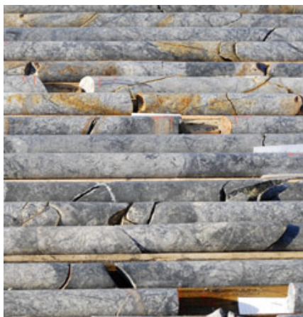
Photo 6. Bottom Coring Samples (USDOI, BOEM, 2013).
