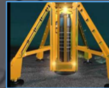
Drilled and grouted pile
