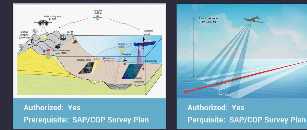
Site-specific surveys conducted to collect information regarding existing resources and conditions above the water, within the water column, and on & below the seafloor. Enables the lessee to characterize existing seafloor and sub-seafloor conditions to select and propose appropriate design, construction, and installation techniques. Results required to be submitted with SAP & COP.
